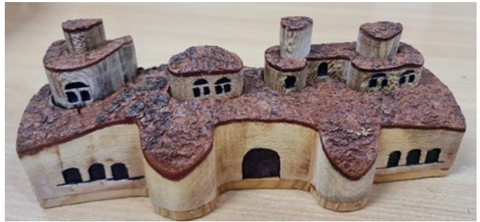
The collapsing Silky Oak castle above was created by Syd Gordon. It is made using a scrollsaw. The saw table is tilted at approx. 1.5 deg to give a slight 'wedge' effect. The pop-up parts are therefore slightly larger at the bottom, so when raising them they wedge into the hole and stay up. They then easily push down to hide them again. It is finished with polyurethane spray.
